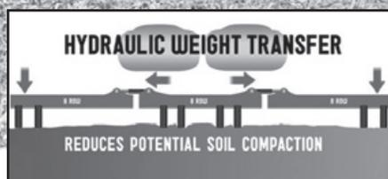
Today's high-volume bulk-fill planters position most of the planter's weight in the middle of the planter bar. Kinze's Hydraulic Weight Transfer system distributes weight evenly across the planter bar, leaving less soil compaction in the center rows and more consistent depth control a the outside rows. That's innovation for planting in the real world.
